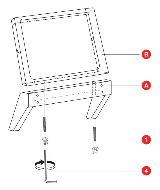
Attach the seat cushion (C) to the wood leg (A) by using 5/16 x  $2\frac{1}{4}$  L bolts with washers (3) and tighten using 3" x  $1\frac{1}{4}$ " L allen key (4).
