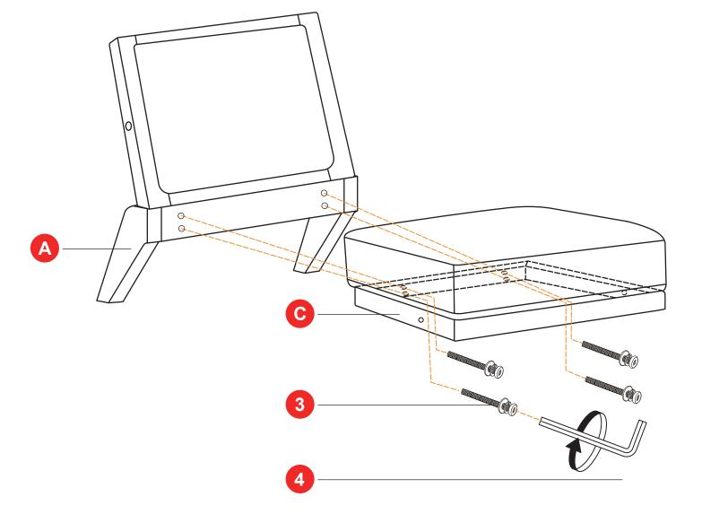
Attach the left and right arm frame (D & E) to the seat cushion (C) by using 5/16" x  $2\frac{1}{4}$ " L bolts with washers (3) and tighten using 3" x  $1\frac{1}{4}$ " L allen key (4).
