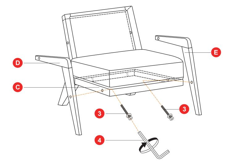
Attach the left and right arm frame (D & E) to the back frame (B) by using 5/16 x  $2\frac{1}{2}$  L bolts with washers (2) and tighten using 3" x  $1\frac{1}{4}$ " L allen key (4).
