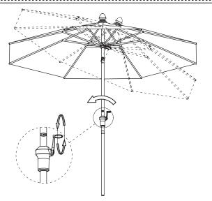
A. Slowly rotate the crank handle counter-clockwise to make the top of umbrella level.
