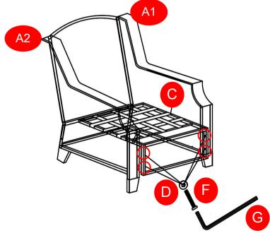
Secure seat panel (C) to assembled chair back (B) with 2 washers (D) and 2 screws (F) by using allen wrench (G). Verify the alignment and adjust, then fully tighten all the screws.
