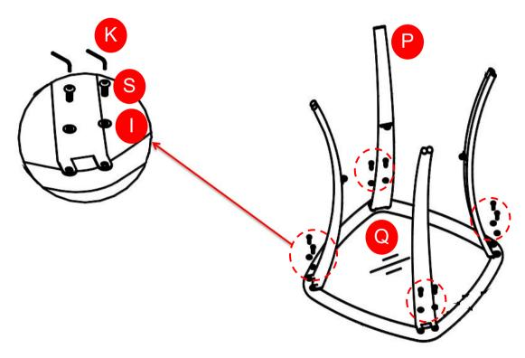
Secure table tray (R) to 4 table legs (P) by using 4 screws (S) and 4 washers (I) with allen wrench (K). Do not fully tighten all screws now.
