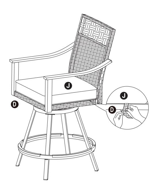
Put the Cushion (J) on Seat Board (D), tighten the fabric band on both side.
