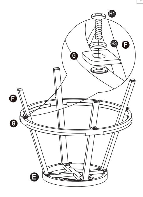
Assemble the Footrest Cover(G) to Chair Leg(F) with Bolt (H1) and Flat Washer (H3), tighten all the bolts to 80% degree with Allen Key(HW1).
