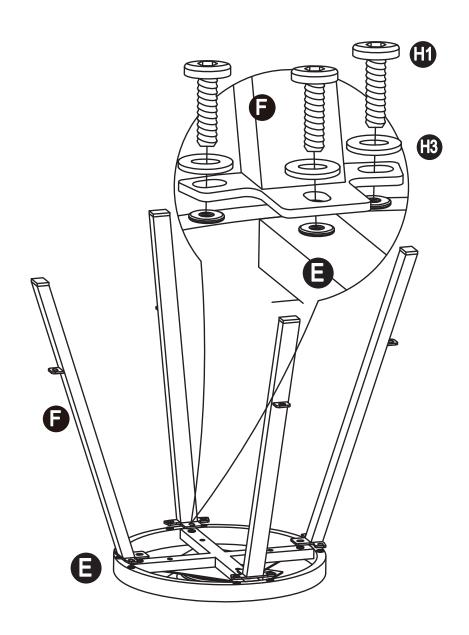
Assemble the Chair Leg(F) to Turnplate (E) with Bolt (H1) and Flat Washer (H3), tighten all the bolts to 80% degree with Allen Key(HW1).
