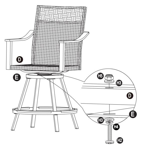
Assemble the Seat Board (D) to Turnplate (E) with Bolt (H2),Nut(H5),Spring Washer(H4) and Flat Washer (H3), tighten all the bolts to 100% degree with Allen Key(HW1). tighten all the Nuts to 100% degree with Wrench (HW2).
