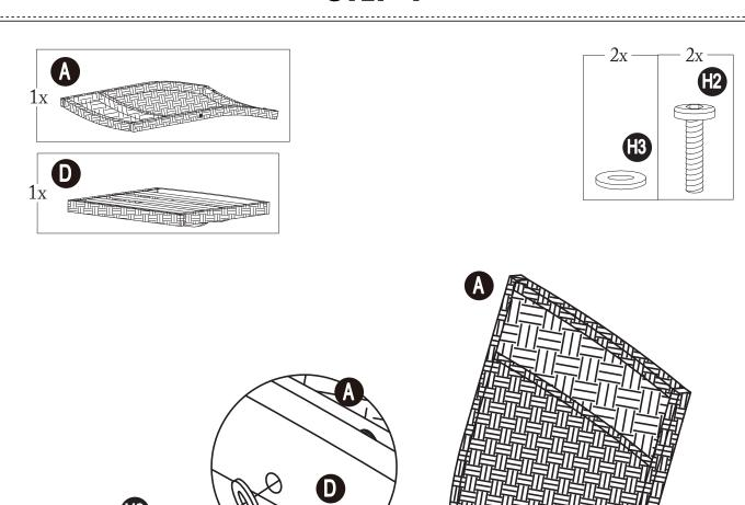
Assemble the Chair Back (A) to Seat Board (D) with Bolt (H2) and Flat Washer (H3), tighten all the bolts to 80% degree with Allen Key (HW1)
