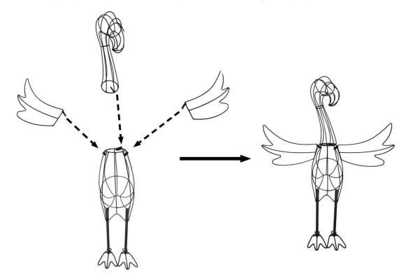
4. Secure the installing points with plastic ties and secure the base to the soft ground by fully inserting 2 stakes into the ground.
