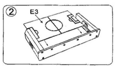
Insert the playing surface (E3) into groves of the assembled pieces from step 1 as shown.
