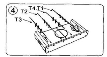
Install the bars (T1,T2,T3 & T4) into the pre drilled holes along the long board.
