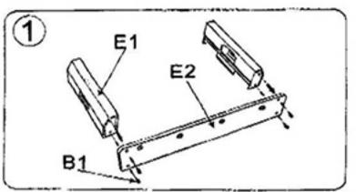
Use 4 screws (B1) to attach two short boards (E1) and one long board (E2) with wrench (included)
