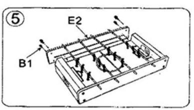
Position the remaining long board (E2) and attach securely as in step 1
