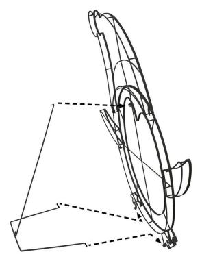
5. Insert the prongs of the Red stake (G) into the corresponding rings on the Y (H).
