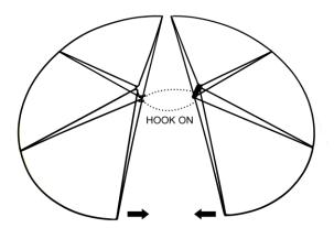
3. Insert the bigger tip of Lower pole (B) into the middle of the hole of Base (A). Snap the hole on the Base (A) with the cap on the Lower pole (B).
