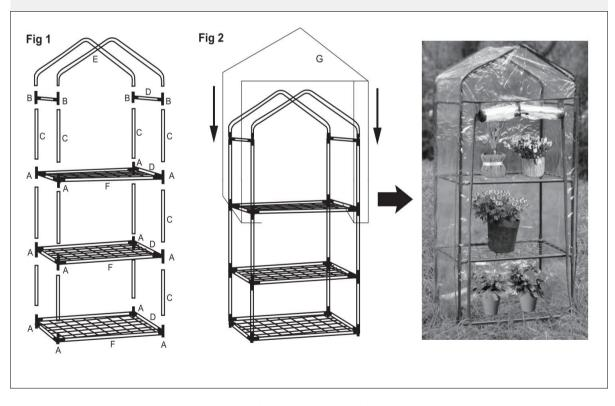
Once assembled, slide the Cover (G) over the frame and secure with ties in the bottom.
