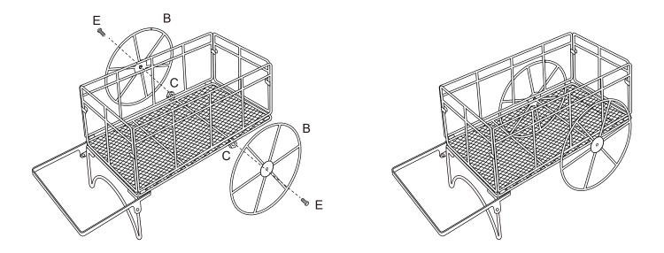
Step 2. Instal the Metal wheels (B) to the Metal basket(A) by Nuts (C) & Large screws, and please put parts as illustration shows.
