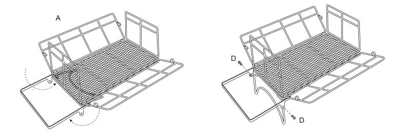
Step 1.Firstly, Assemble Metal basket (A) as illustration shows. Then, fasten Metal basket (A) by small screws (D).
