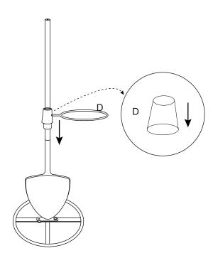
Step 4. Insert Planter hoop (D) to the tube as illustration shows. Please note that the large side should be down.
