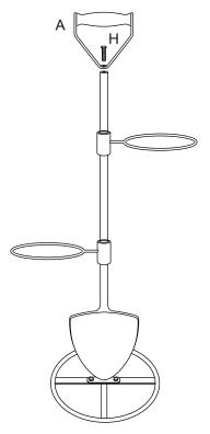
Step 6. Assemble Wooden handle (A) to the Upper tube (B) as illustration shows, and tigthen screws by Hex wrench (J).
