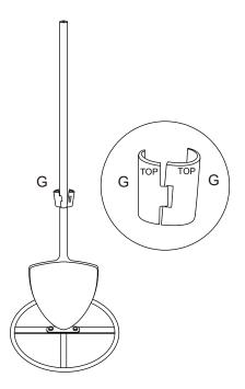
Step 3. Put the Plastic retaining buckle (G) to the tube as illustration shows.
