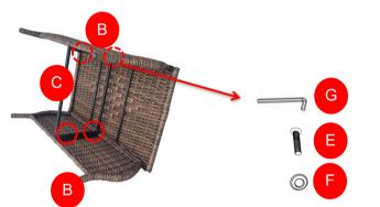
Secure 2 table side boards (B) to table top (A) by using 4 short Secure table support frame (C) to 2 table side board (B) by using 4 screws (E) and 4 washers (F) with allen wrench (G). Do not fully tighten screws now.
