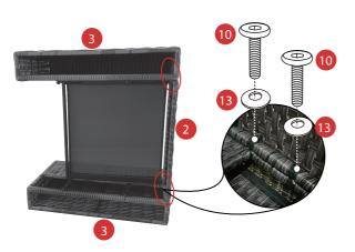
PARTS REQUIRED: 1, 3, 10, & 13 Keep the bolts loose.
