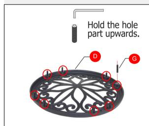
Secure 8 bolt (G) into chair seat (D) by using allen wrench (M). Do not fully tighten all screws now.
