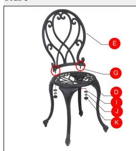
Secure chair back (E) to chair seat (D) with 2 bolt (G), 2 washer (I), 2 spring washer (J) and 2 nut (K) by using allen wrench (M) and open end wrench (N). Do not fully tighten all screws now.
