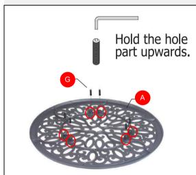
Secure 6 bolt (G) into table top (A) by using allen wrench (M) . Do not fully tighten all screws now.
