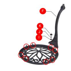
Secure 4 chair legs (F) to chair seat (D) with 8 washers (I), 8 spring washers (J) and 8 Nuts (K). Do not fully tighten all screws now.
