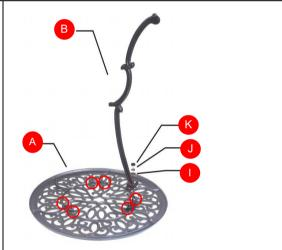
Secure 3 table legs (B) to table top (A) with 6 washers (I), 6 spring washers (J) and 6 nuts (K). Do not fully tighten all screws now.
