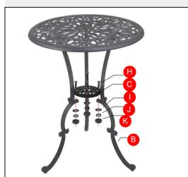
Secure table support (C) to 3 table legs (B) with 3 screw (H), 3 washer (I), 3 spring washer (J) and 3 nut (K) by using allen wrench (M) and Open End Wrench (N). Do not fully tighten all screws now.
