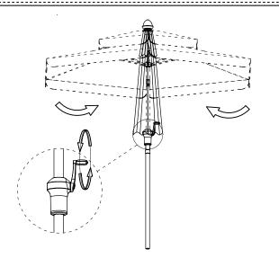
A. Rotate the crank handle counter-clockwise to close the umbrella
