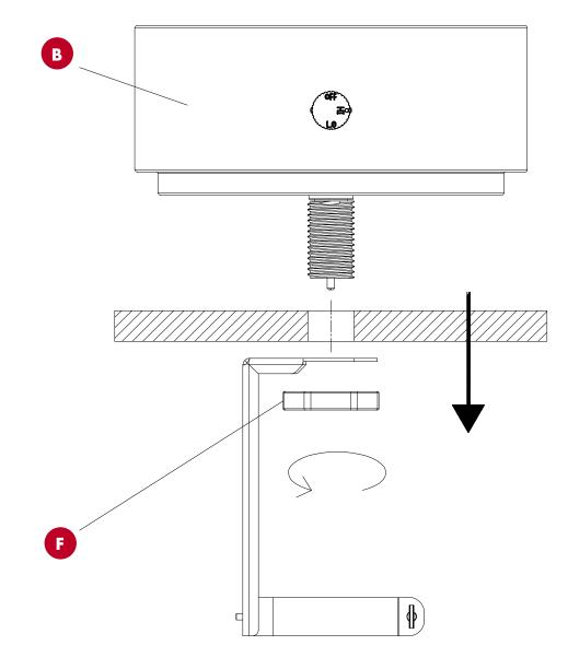
Check that the control knob (C) for the gas supply system is turned to the "OFF" position before assembling the 1 lb. propane gas tank. To attach the 1 lb. propane gas tank (not included) on the unit, screw the 1 lb. gas tank to the regulator inlet fitting.
