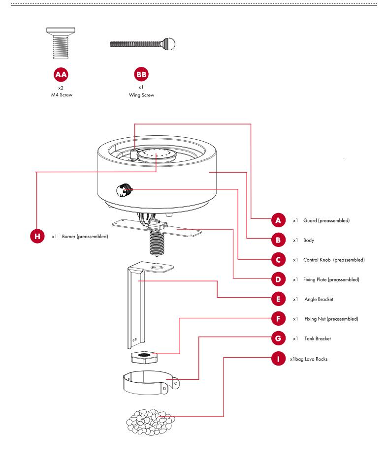
Unscrew and remove the fixing nut (F) from the threaded post.
