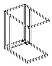
Insert Leveler (3) into the Lower Support Frame (B) and fully tighten. Return the table to the upright position. The levelers can be adjusted as needed so the Table is level and stable. All adjusters should be in full contact with the floor.
