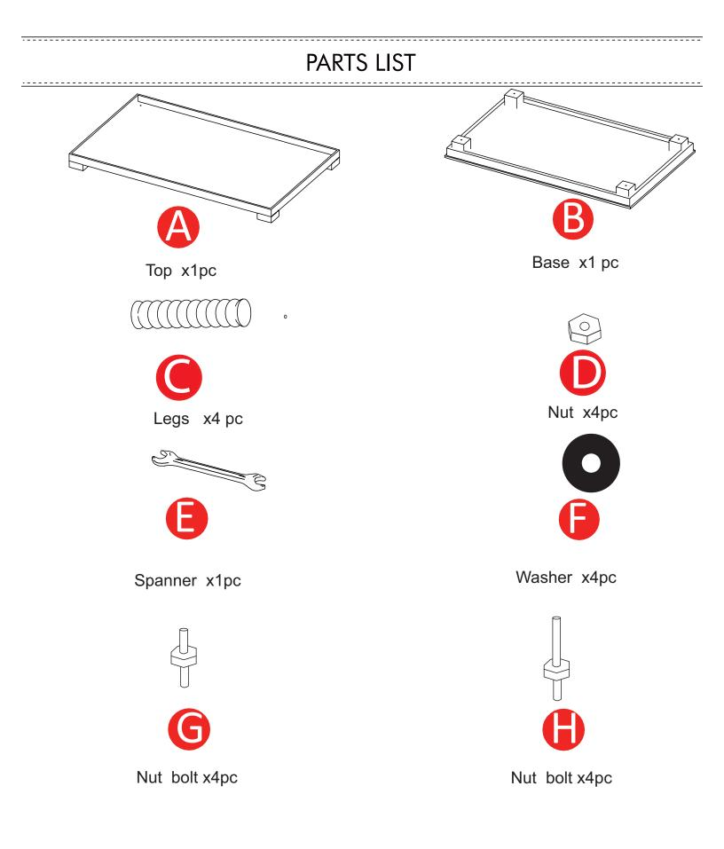
1.Align the holes in the end of Legs (C) with the Nut Bolts (G) in Top (A). Turn the legs (C) in a clockwise direction until fully tightened.
