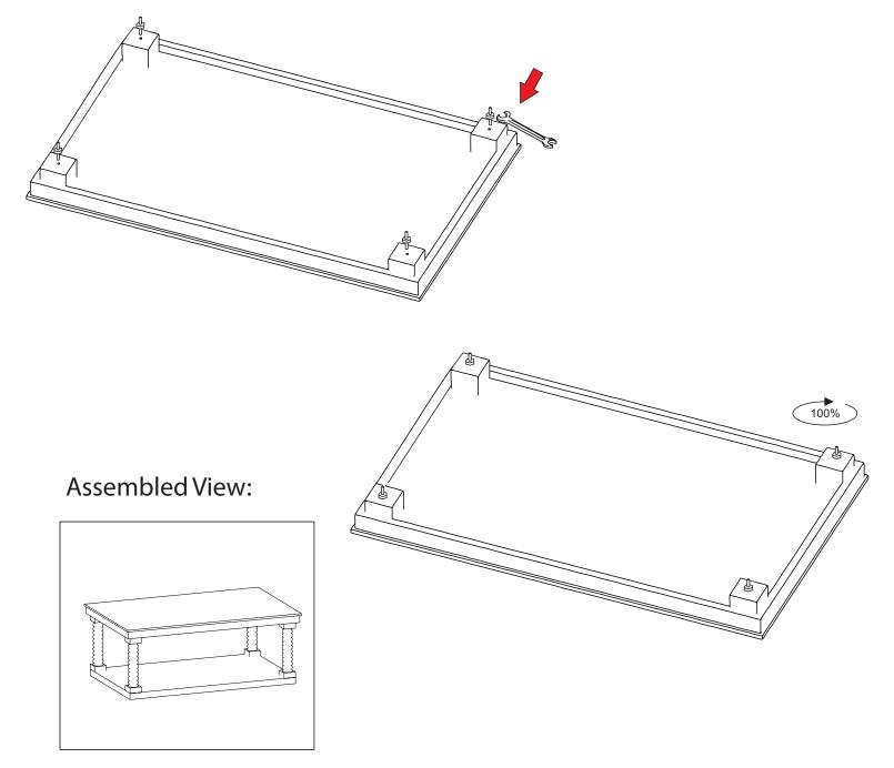
1. Align the holes in the end of Legs (C) with the Nut Bolts (G) in Top (A). Turn the legs (C) in a clockwise direction until fully tightened
