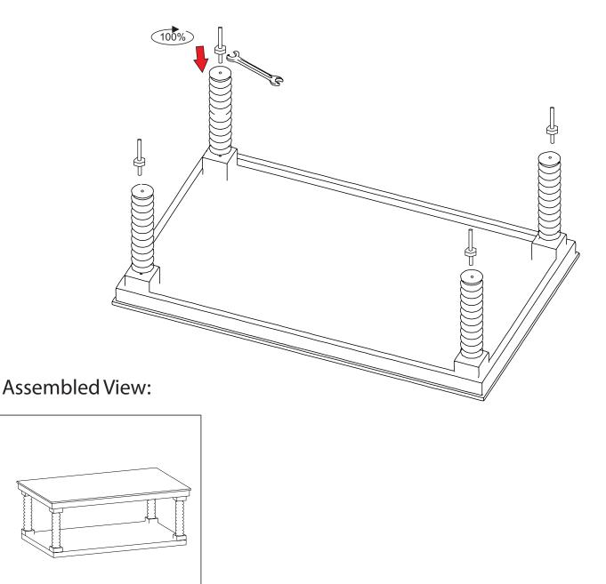
1. Align the holes in Base (B) with the Nut Bolts in Legs (C) and lower into place.
