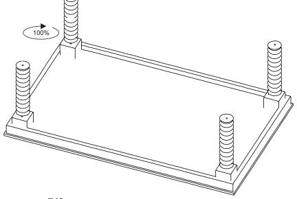
1.Tighten Smaller Side Nut Bolt (H)Legs(C)clock wise 100%By help of Spanner(G).
