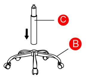
Insert part (C) into the center hole of part (B) as shown in the diagram.
