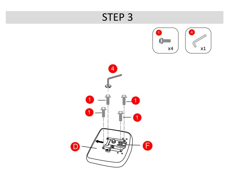
Align the holes in part (D) with the holes in part (F). Using screws (1) and Allen Wrench (4), attach part (F) to part (D) as shown in the diagram. Fully tighten all screws.
