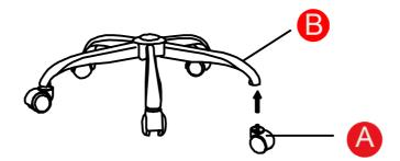
Insert the part (A) into part (B) as shown.
