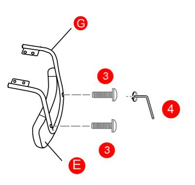
Align the holes in part (G) with the holes in part (E). Using screws (3) and Allen Wrench (4), attach part (G) to part (E) as shown in the diagram. Fully tighten all screws.
