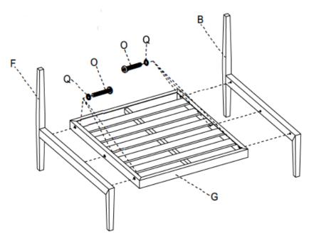
Step 6 Attach Armless Back Panel (H) to Left Leg (B) and Right Leg (F) and Armless Seat Panel (G) by using 4 washers (Q) and 4 short Bolts (P).
